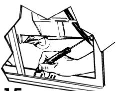
Check door for proper operation. Door should close easily without slamming and open with its own weight. If necessary, close door and adjust both door springs by moving spring ends to different holes in base.
